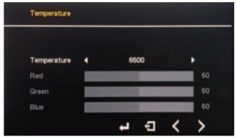
**-Temperature**: Adjust the tint of screen to 9300k, 7500k, 6500k, 5800k, sRGB, User.
