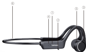
①LED indicator light ②Charging port ③Microphone ④MFB(Multi-function button) ⑤Bone conduction vibrator ⑥Silicone memory neckband
